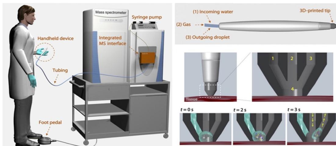
Figure 8. Schematic representation of the MasSpec Pen system and operational steps. The tip contacted the tissue for analysis, where the vacuum and the gas conduits were concomitantly opened (arrows) to transport the droplet from the MasSpec Pen to the mass spectrometer through the tubing system for molecular analysis. Reproduced with permission.<sup>[21]</sup> Copyright 2017, American Association for the Advancement of Science.
